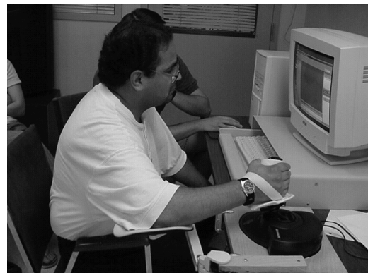
Figure 1: Prototype web-based, force feedback telerehabilitator ("Java Therapy")
