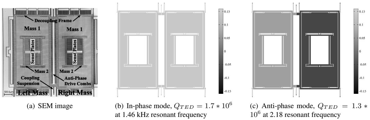
Figure 1: (a) SEM of the bulk micromachined anti-phase driven vibratory gyroscope with multi-DOF sense-mode. (b,c) COMSOL FEM of thermoelastic damping (colors represent x-displacement).
