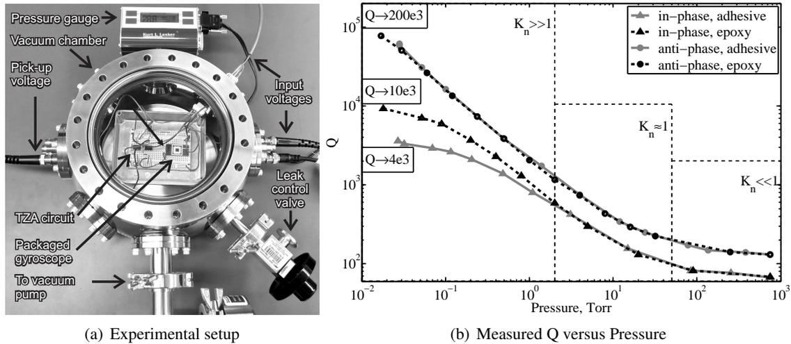
Figure 2: Experimental measurement of quality factor  $Q$  for the in-phase and anti-phase modes. “Epoxy” and “adhesive” stand for the die attachment techniques using CircuitWorks conductive epoxy and SPI conductive double sided carbon adhesive tape respectively.  $K_n$  is the Knudsen number and is calculated assuming  $5 \mu\text{m}$  characteristic gap.
