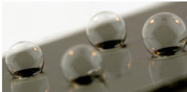
Fig. 3. Fabricated array of hollow micro glass spheres.
