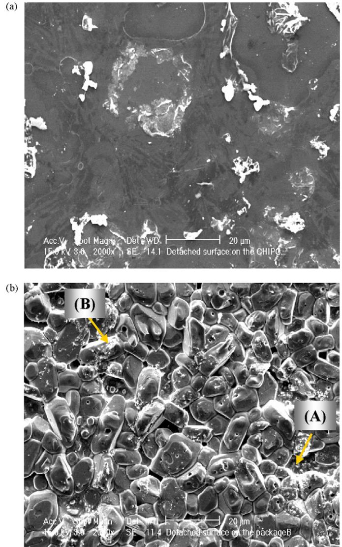
Fig. 2. SEM images of a sample bonded with  $320^\circ\text{C}$  processes: (a) detached Si chip (b) detached alumina substrate.
