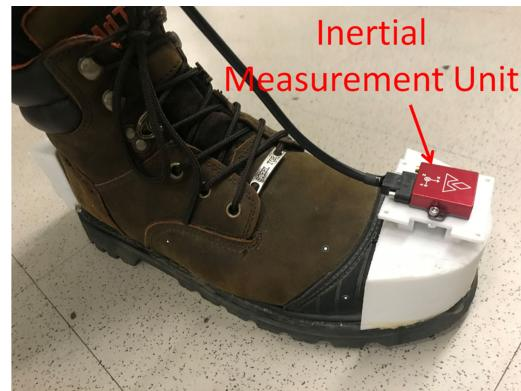
Fig. 1. Foot-mounted IMU used in ZUPT-aided pedestrian inertial navigation. A near-tactical grade VN-200 IMU was rigidly mounted above the forefoot of the boot by three-dimensional-printed fixtures for better navigation accuracy [4].
